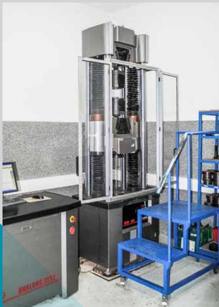
The tests are carried out according to the specified standard on two machines that can measure the force in the range of 0 - 600kN.
